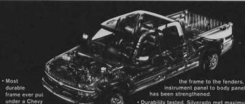
· Three-piece modular frame whose front section is made from hydroformed steel.
